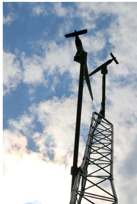
Anemometers at 6m and 10m record different wind directions.
