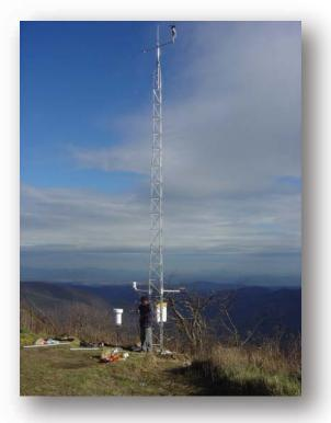
emergency maintenance. The station located at Mt. Mitchell collapsed due to heavy ice and wind in September. The station has been repaired and is back functioning as of early March.
